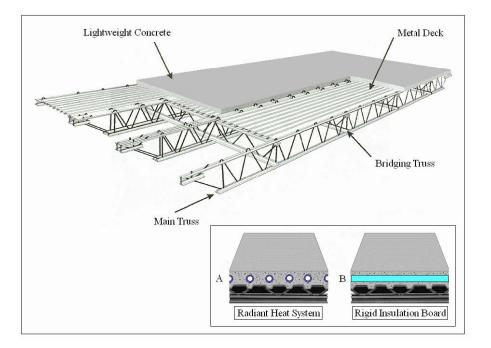
Application for insulated properties as well as a sound barrier for lightweight composite roof or floor deck in commercial, industrial, residential buildings/structures. This would especially true for power utility problems currently being experienced in hot and cold regions where electricity, gas or oil consumption is an issue. Heating and cooling costs are reduced.
